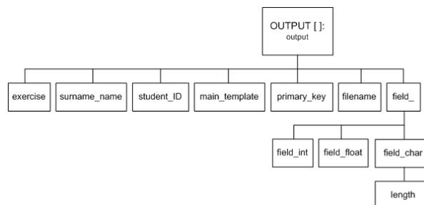
Figure 4: Specification diagram of student's exercise generator
