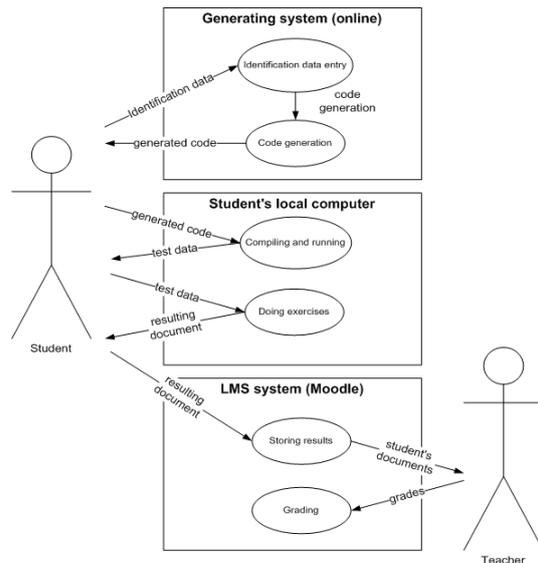
Figure 7: Use-case diagram of the generation system
