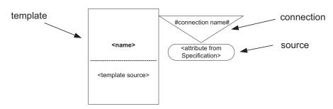
Fig 7: Elements of Configuration Diagram
